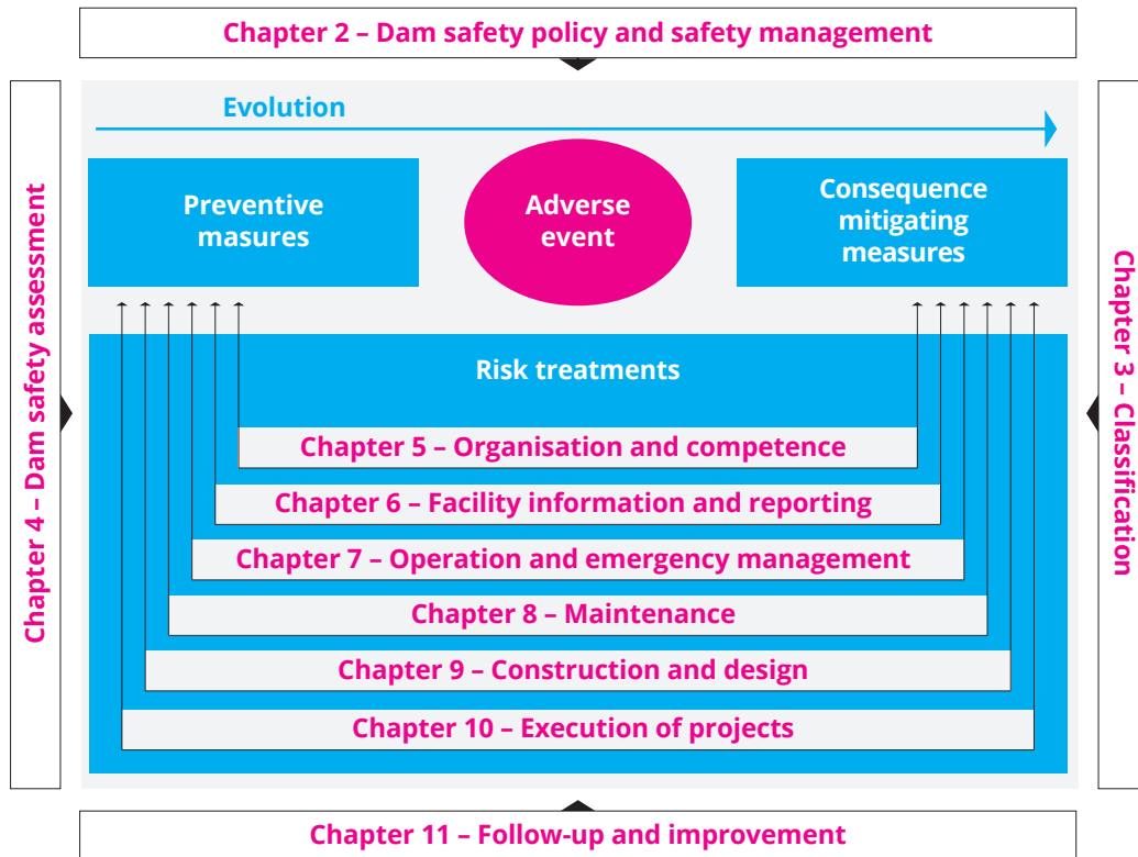
Figure 1. RIDAS structure with risk treatments for a dam facility in the inner box, as well as general conditions, classification, dam safety assessment and follow-up.
